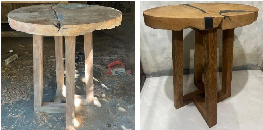
Gambar 1. Warna kayu sebelum proses ebonisasi (kiri) dan sesudah proses ebonisasi (kanan) Figure 1. Wood color before ebonization process (left) and after ebonization process (right)
